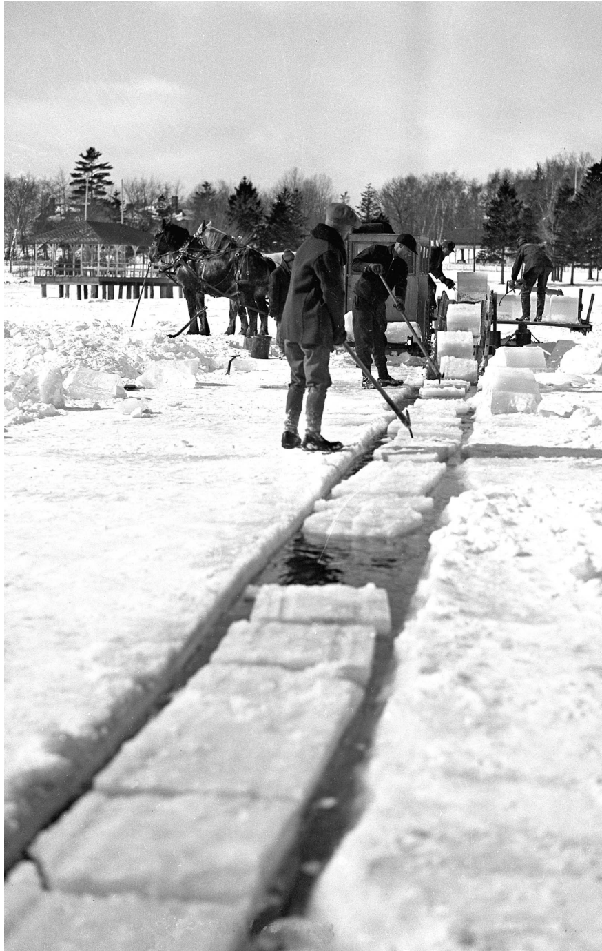
Ice is guided with pike poles to a conveyor belt that will hoist them up onto a horse-drawn sledge, sometimes as fast as one per second. Photo take just off Depot Beach.
