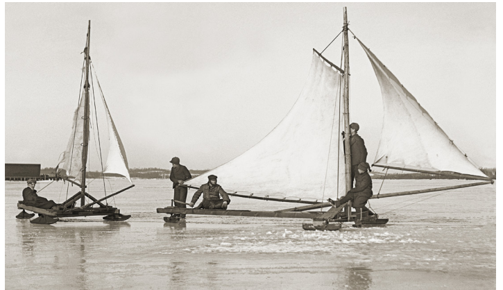
Two iceboats about to be unleashed on a frozen Lake Charlevoix. Said to be able to reach ninety mph with only a fifteen mph wind behind it, under perfect conditions a well-built iceboat was sometimes capable of reaching Boyne City in ten minutes.
